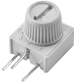
The Model 63 cermet trimmer manufactured in Europe is readily available in several pin configurations for top or side adjustment and with a choice of Knob styles for finger setting. Quick adjustment is achieved with multi finger wiper and the standard resistance range is between 10Ω and 2 MΩ with a tolerance of ± 10%. This sealed (IEC 68-2-17) single turn trimmer is continuing to provide excellent performance as the industry standard across a broad spectrum of applications.
